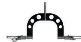
MEASUREMENT BY TRAIN WHEEL
